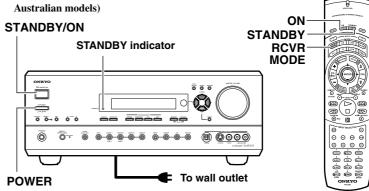
Turning on the power may cause a momentary power surge, which might interfere with other electrical equipment on the same circuit, such as computers. If this happens, use a wall outlet on a different circuit.
